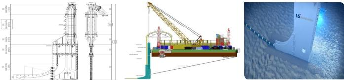
The Vertical Injector is a highly modular and adjustable vessel or barge mounted sub-sea burial tool, capable of burial depths up to 10 meters under the seabed.
